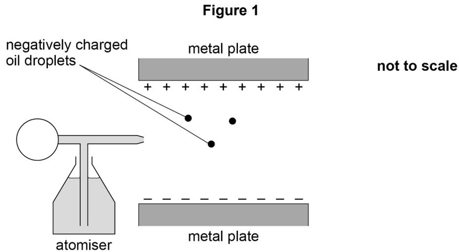
Negatively charged oil droplets are sprayed from the atomiser into the gap between the two horizontal metal plates. A potential difference is applied between the metal plates.
